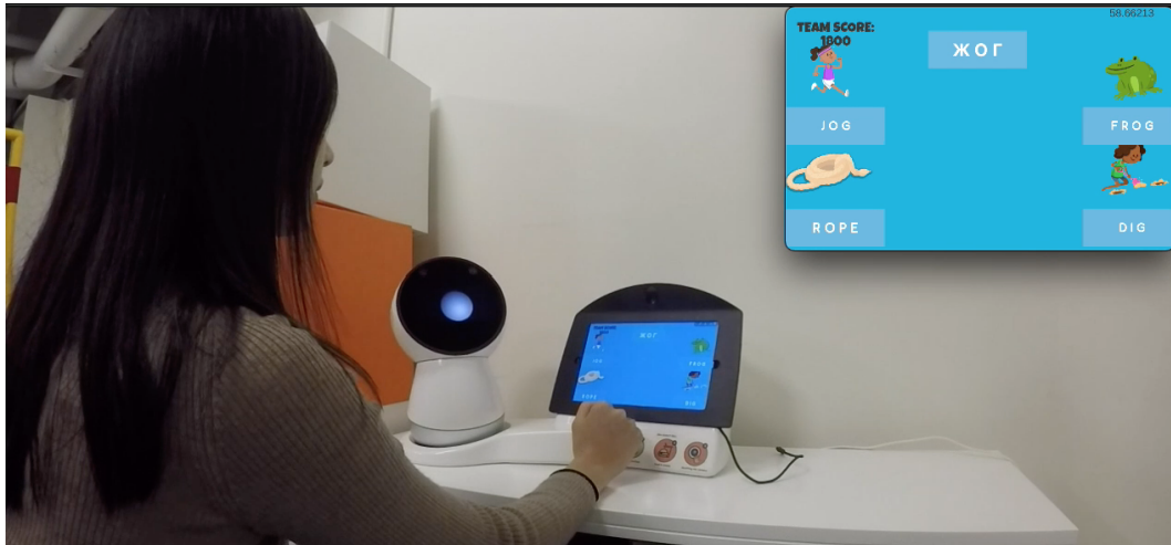
Figure 18: GoPro camera view for human subjects study. Setup includes front-facing camera within Station, microphones inside Jibo robot, Android tablet screen-recording, and a GoPro camera.
