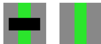
Figure 9. On the left the image to inpaint ( \Omega in black); on the right the inpainted result ( 2L + 1 = 3 , l = 1 ). Our algorithm guarantees the connectivity principle, whatever is the size of \Omega (result according with [34]).
