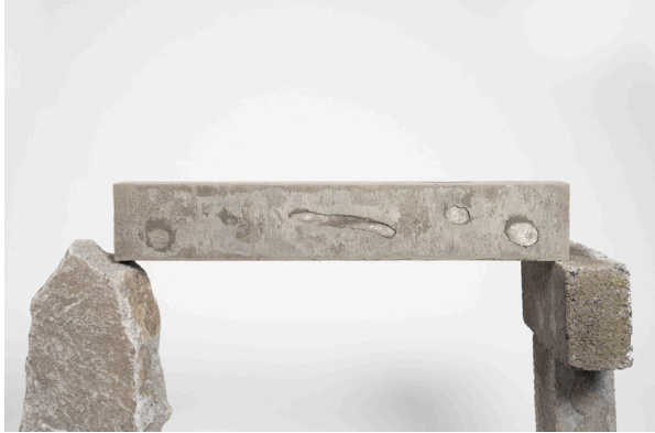
Figure 5.2.5. Locally material removed topology optimized beam - Before erosion: This image depicts the beam prior to the removal of the gypsum material
