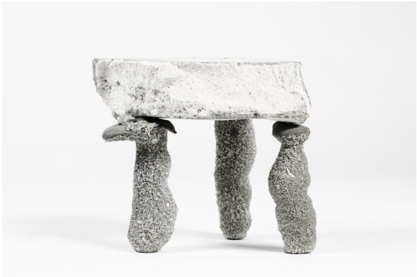
Figure 5.3.10. Geomorphic dolmen: The slab was positioned on top of injection 3D printed columns using a dolmen construction technique.
