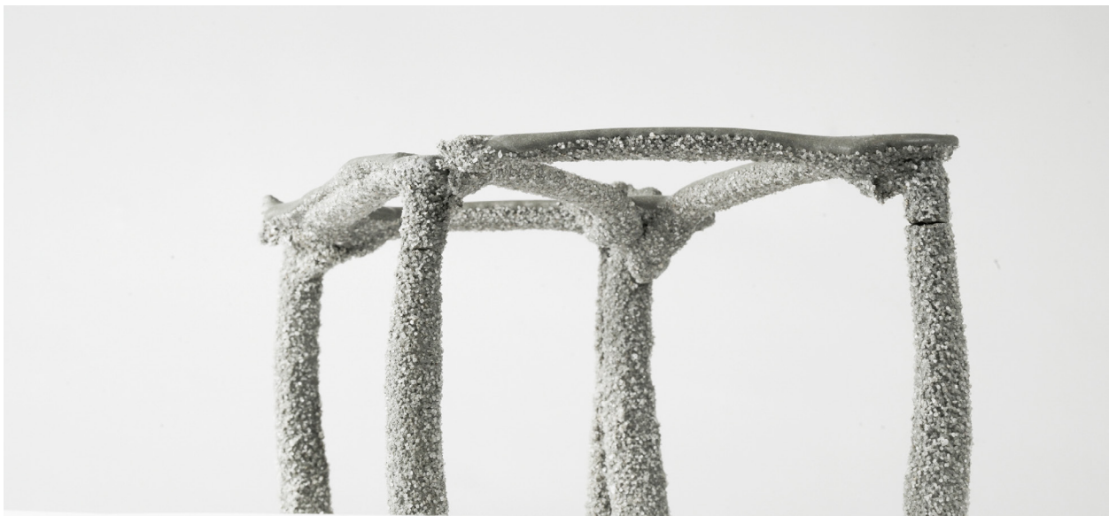
Figure 5.3.4. A sequence of gravity demolding: Once the sandbox is taken apart, the sand falls from the concrete structure due to the force of gravity.
