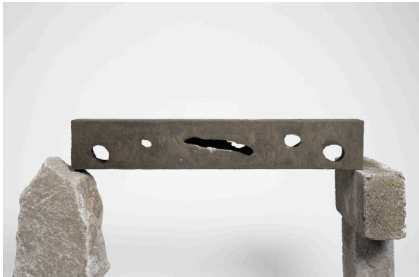
Figure 5.2.6. Locally material removed topology optimized beam - After erosion: This image illustrates the result after the gypsum was exposed to water and eroded away. The gypsum mixture was specifically injected in areas where the generative design determined that the material was unnecessary. The beam could be fabricated to express an optimized design or hidden inside the prismatic shape.
