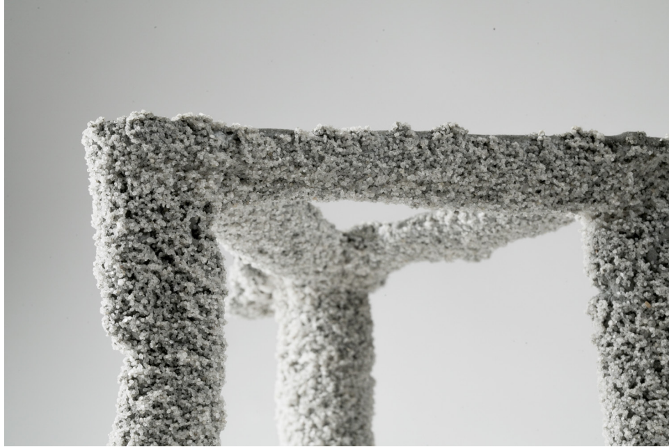
Figure 5.3.11. Geomorphic concrete frame structure: Close-up picture of a concrete structure fabricated from injection 3D concrete printing into sand.
