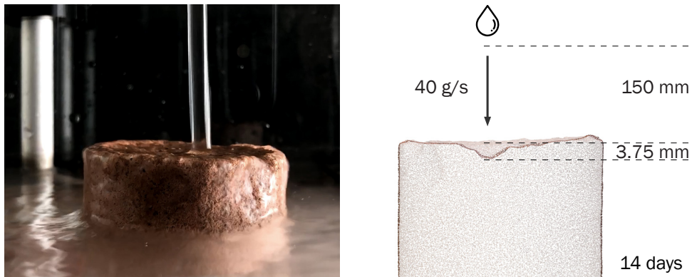
Figure 4.3.7. Erosion test - GYP-230414-2: After a 14-day test, a specimen's surface exhibits a pavement depth of 3.75mm. The image on the right represents the pavement from 3D scanned model.
