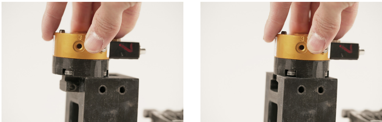
Figure 4.2.11. Connection detail for easy tool change: The tool's connection mechanism is specifically crafted for effortless mounting and dismounting from the 6-axis robot arm. It is possible to change tools by simply inserting the tool into the duck-tail joint host, which is linked to the robot arm.
