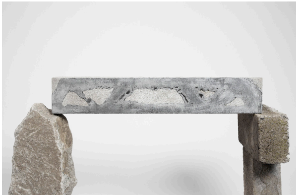
Figure 5.2.4. Locally reinforced topology optimized beam: The darker sections of the beam are injected with high-strength concrete, while the brighter portions are cast with lightweight concrete. Unlike formwork methods, the material used for injection 3D printing is not wasted but remains within the injected concrete.
