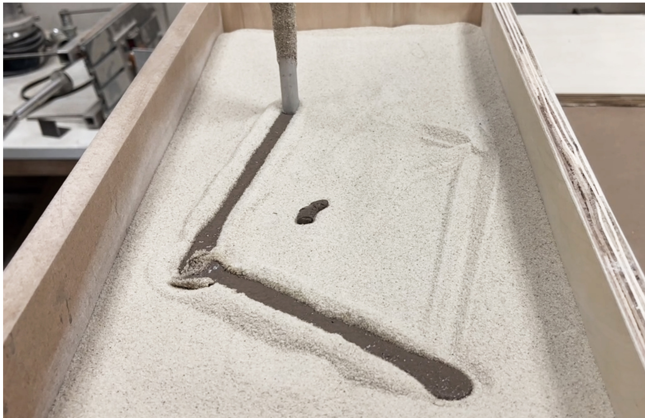
Figure 5.3.3. Inject 3D concrete printing into the sand: A nozzle connected to the extruder traverses through the sand and dispenses concrete. This single-stroke fabrication is inspired by Edison's invention and the geological formation process of column structures found around Crowley Lake.
