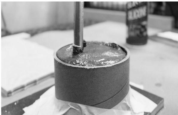
Figure 4.4.2. Injection 3D printing in tube mold: Injection 3D printing gypsum mixture into the liquid concrete with a 5mm inner-diameter nozzle.
