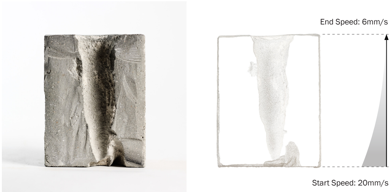
Figure 4.4.6. Injection 3D print with various widths: Left picture displays the gypsum injection captured in a concrete cut, while the right image shows a cross-sectional view of a 3D scan of the same object. The extrusion process begins by depositing gypsum from the base and moves upwards, with the retraction speed altering. The nozzle used has a diameter of 9mm, and it initially moves at a speed of 20mm/s. The speed gradually reduces at a rate of 0.14\text{mm/s}^2 until it reaches a final tool path speed of 6mm/s.
