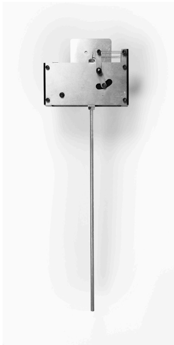
Figure 4.2.6. Metal cable extruder: This tool extrudes a 3/32" diameter cable into liquid concrete.
