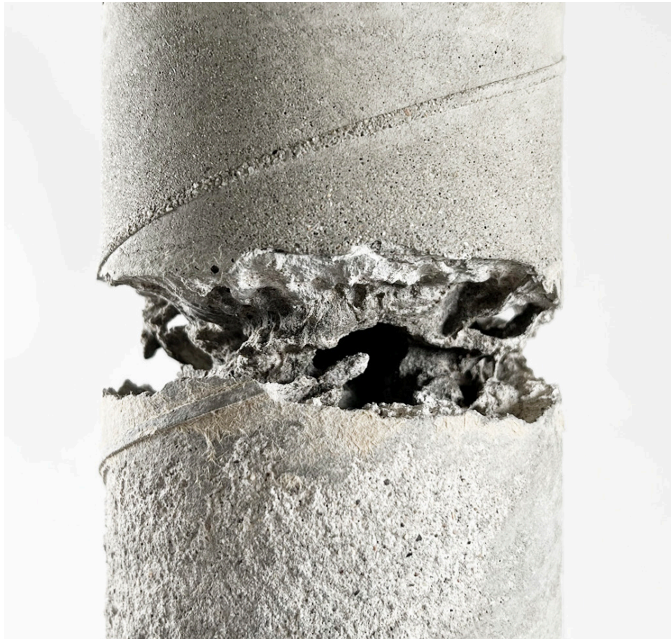
Figure 5.4.9. Locally eroded geomorphic concrete column: By locally injecting a gypsum mixture, it is possible to create shapes and patterns that resembles the structure of a cave on a cylindrical surface.
