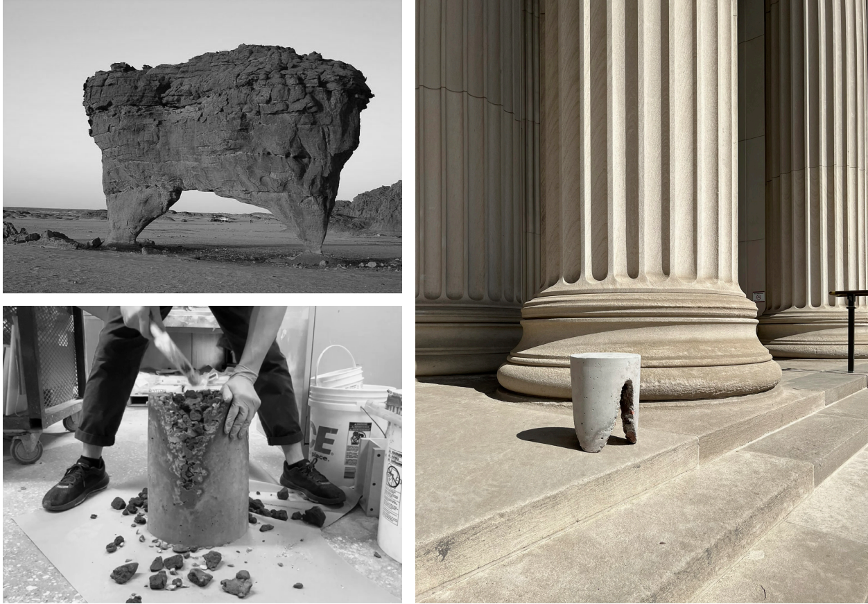
Figure 3.3.2. Eroding Stool: Rock-jammed formwork was used to fabricate a concrete stool. Jammed rock falls and erodes with time. This design draws inspiration from an arch-shaped standing rock in the desert formed by the eolian process (Bottom-Left, Right). Standing rock in Tassili n'Ajjer, Algeria - Reprinted from picstatio.com, 2017 (Top-Left).
