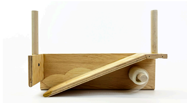
Figure 4.2.4. Concrete Pour-inter: Hand 3D concrete printing and fiber reinforcement tool that is inspired by wood plane, and Urschel's machine.
