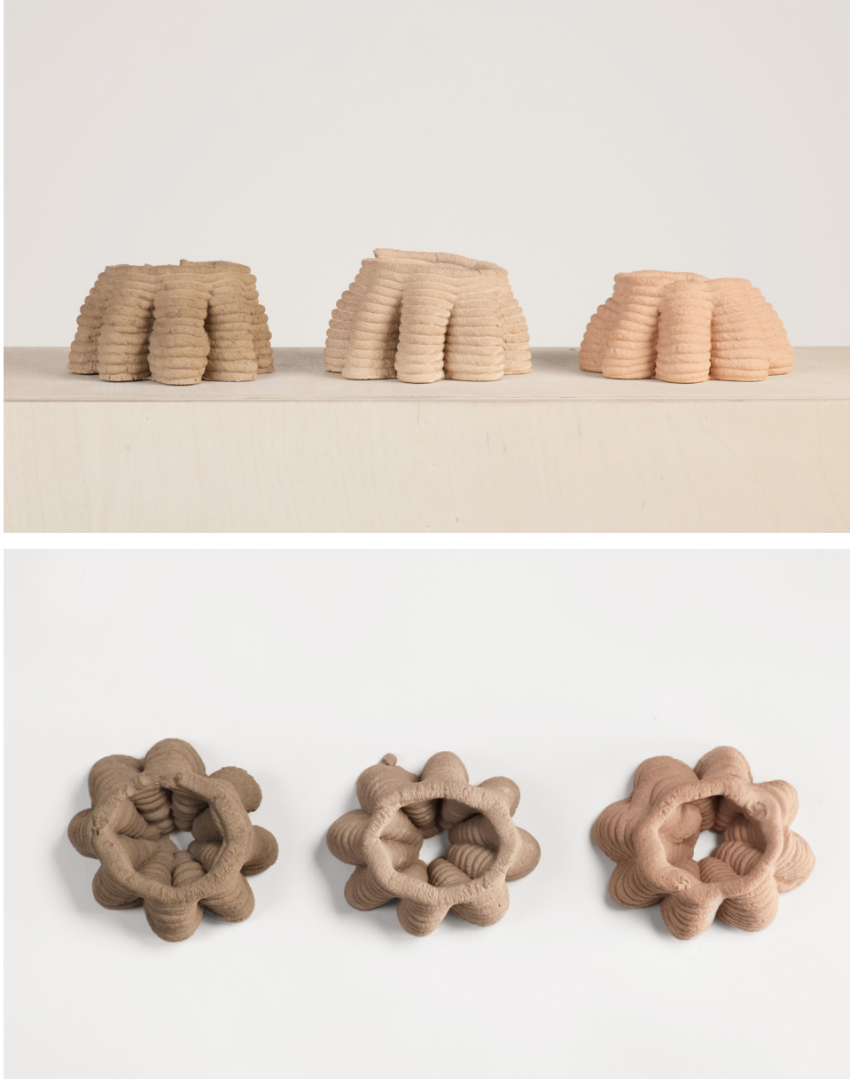
Figure 4.3.5. Printability test: Extrudability and buildability test for gypsum mixture.
