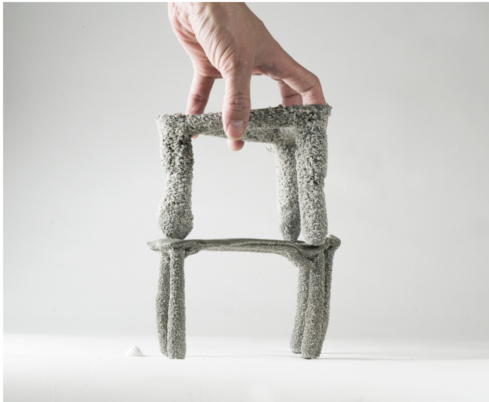
Figure 5.3.13. Geomorphic concrete tall structure: By stacking sandboxes based on the extending injection printing height, it is possible to construct taller structures.
