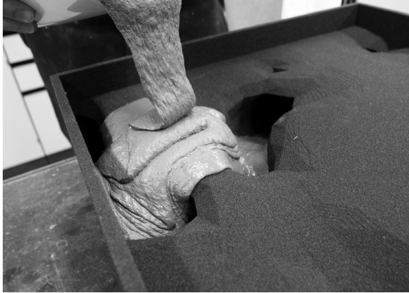
Figure 3.1.2. 3D printed Formwork: Digital Building Technologies in ETH developed hybrid of 3D printing and conventional casting fabrication method - Reprinted from Jipa & Dillenburger, 2022.
