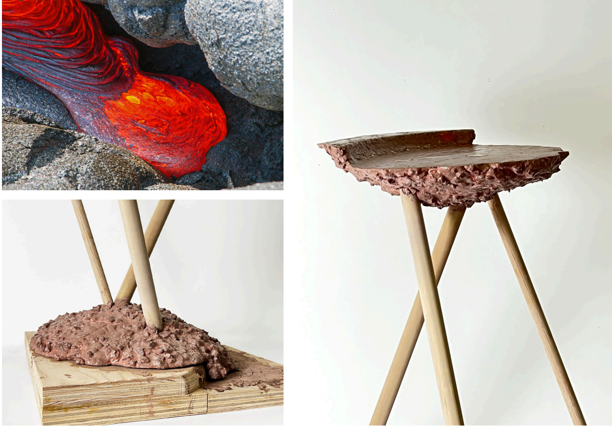
Figure 3.3.3. Flowing Stool: The stool is formed as the liquid concrete sets and hardens, a process that draws inspiration from the transformation of flowing magma into igneous rock (Bottom-Left, Right). Flowing magma from Hawai'i volcanoes national park - Reprinted from bigislandhikes.com, 2017 (Top-Left).
