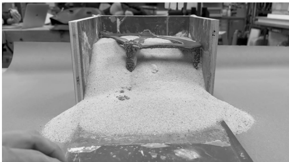
Figure 5.3.4. A sequence of gravity demolding: Once the sandbox is taken apart, the sand falls from the concrete structure due to the force of gravity.
