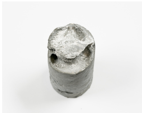
Figure 4.4.7. Spiral cavity: A spiral-shaped cavity was formed inside a concrete cylinder by injecting and printing gypsum in a spiral pattern.
