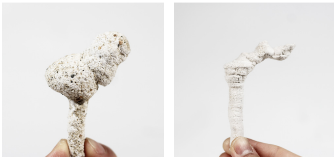
Figure 4.4.5. Intersection point: To ensure the stability of the intersection of more than two prints, additional materials can be extruded. Similarly, the technique can also be applied to secure the point where the tool is turning.
