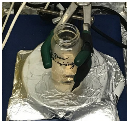
Figure 2.2. The demonstration of the indispensability of air during the synthesis of \text{Co}_3(\text{HITP})_2 . The reaction mixture containing \text{HATP} \cdot 6\text{HCl} , \text{Co}(\text{OAc})_2 \cdot 4\text{H}_2\text{O} , \text{NaOAc} (2 M) in Milli-Q water/DMF is still clear without any precipitate after three-hour stirring under \text{N}_2 atmosphere at room temperature.
