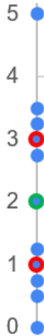
Figure 7. Markers showing the powder layer thicknesses that were tested for the Powder Layer Thickness Test. The minimum and maximum specifications, 1 and 3 units, are highlighted in red. The nominal value, 2 units, is highlighted in green.
