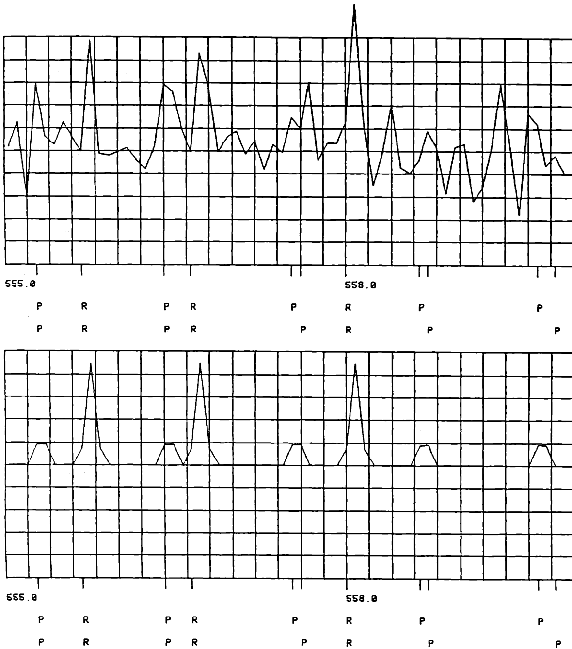
Figure 6.33 ECG Observations with Estimation Results. The upper trace shows the actual signal while the lower trace shows the signal with the Gaussian noise removed. Beneath each trace there are two sets of annotations, of which the upper is true and the lower is estimated.
