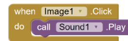
Figure 3: An example where the user changes the functionality of the app, specifically what happens when the image is clicked. Before the edit, nothing happens when the user clicks the image of a dog. The user adds a barking sound and then commands, “When the image is clicked, play Sound1.” The change is represented in the Aptly code and implemented via the creation of new code blocks, as shown on the right.
