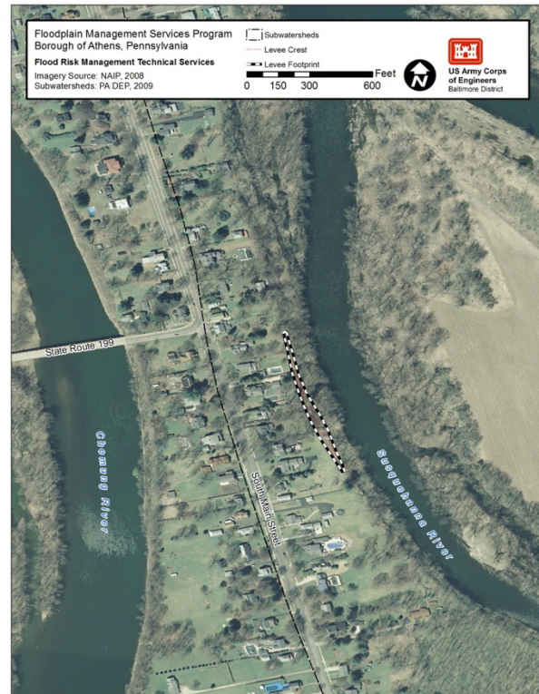
Figure 3: Area 2 Levee Alignment
