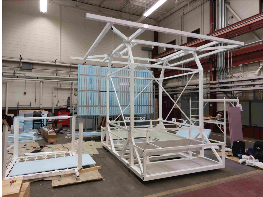
Figure 5-9: The GAPS gondola (large white basket-shaped structure) at MIT Bates prior to integration. The vertical blue foam structure in the back is the cold plate (coupled to methanol chillers) used to cool the radiator during ground testing. Photo courtesy of Brandon Roach.
