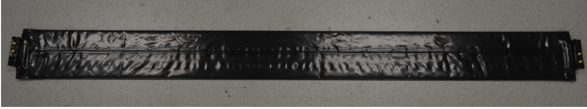
Figure 5-7: A 180-cm-long TOF paddle for the GAPS experiment, wrapped in black vinyl. The SiPMs and preamplifier boards are enclosed in the rectangular structures at each end. Photo courtesy of Takeru Hayashi.
