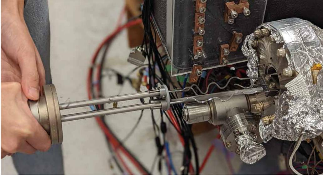
Figure 2-23: The spent and broken titanium filaments replaced during the vacuum chamber maintenance portion of the upgrade. We replaced all three filaments with fresh ones in November 2021.
