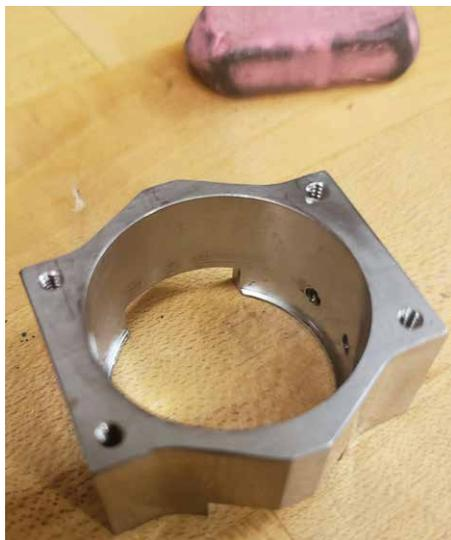
Figure 2-17: The 780nm (lower) lenstube after a layer of Aquadag was removed via friction.
