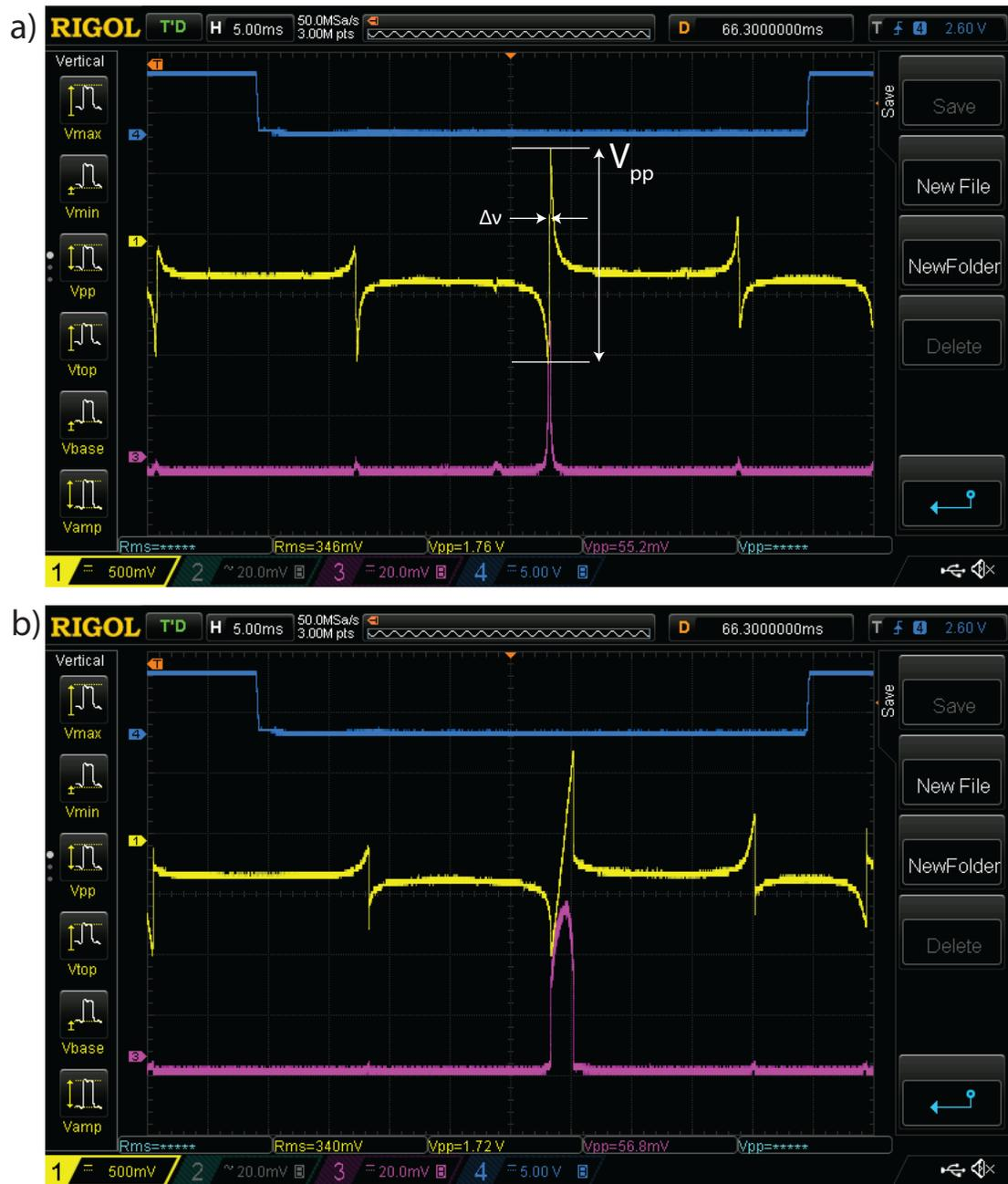
Figure 3-16: The PDH error signal for our installed experimental cavity without (a) and with (b) the fast feedback loop engaged. The sensitivity of the lock can be estimated via the slope of the central feature of the error signal without fast feedback engaged.
