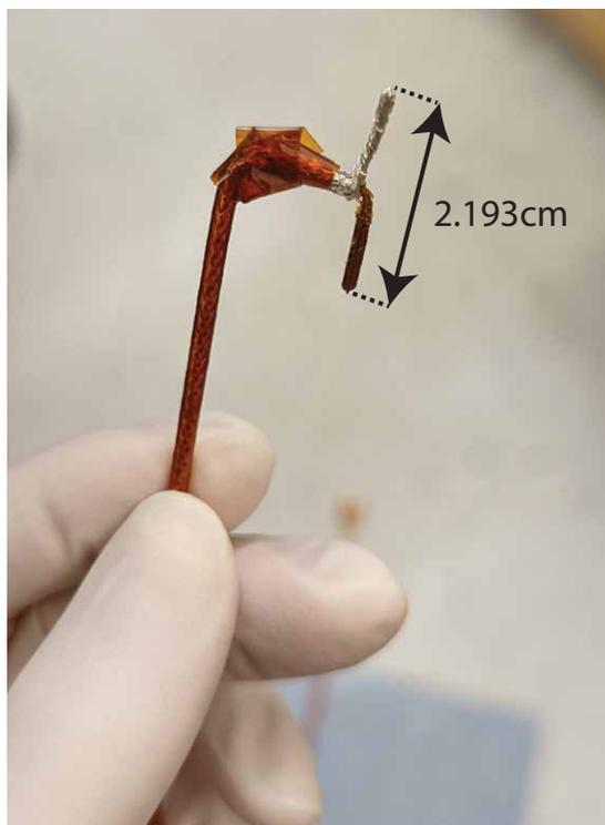
Figure 2-7: Picture of homemade dipole antenna for 6.8GHz transmission.
