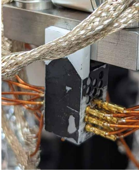
Figure 2-5: One of the Macor Dsub connectors just before the second vacuum installation. The white portion at the top of the Dsub broke off completely from the remainder of the Dsub and was glued back into place using TorrSeal. Looking closely at the areas on the ceramic piece between the separate pins, scrape marks from removing shorts through the graphite coating are visible.
