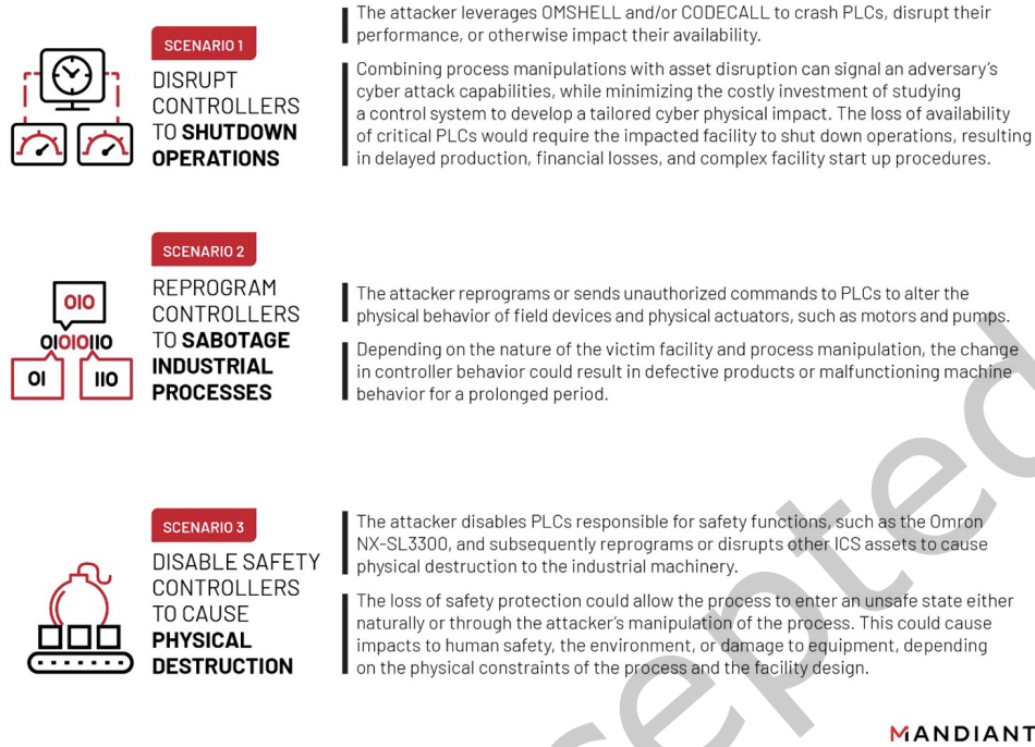
Fig. 11: Three APT Attack Scenarios of the Pipedream Malware (Source: Mandiant)
