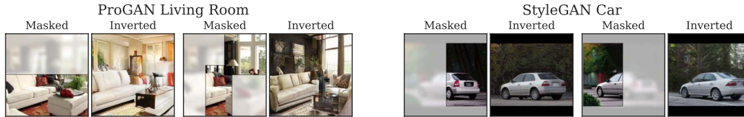
Figure 3-2: Image completions using the latent space regressor. Given a partial image, a masked regressor realistically reconstructs the scene in a way that is consistent with the given context. The completions (“Inverted”) can vary depending on the exposed context region of the same input.
