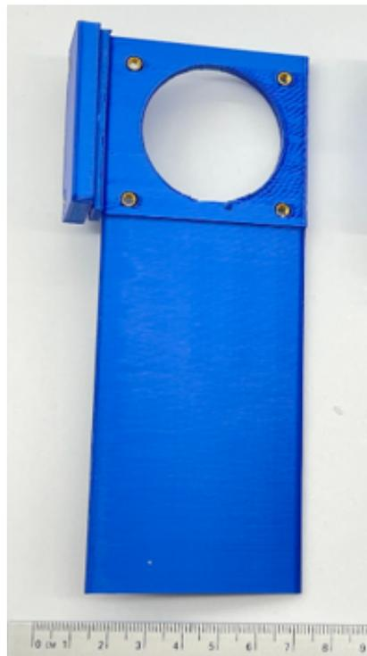
Figure 21. This is the fan frame with hood to help prolonged concentration of the cooled on the fiber length.
