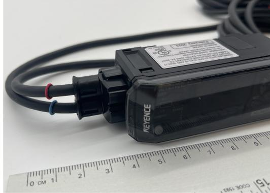
Figure 49. This shows the IG-1000 amplifier with its connection to the receiver (red strip) and the receiver (blue strip).
