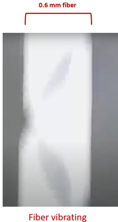
Figure 40. This shows the instability of the fiber when looked through the microscope lens causing the diameter to increase to 0.6 mm.
