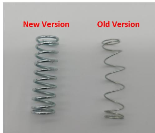
Figure 98. This shows the spring from the previous design and the new stronger spring to aid in alignment and prevent slippage of the preform.
