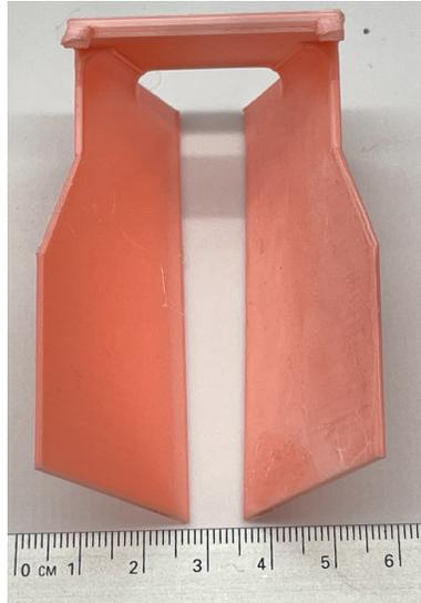
Figure 10. This is the hood that is attached to the axial fan to help concentrate the cooled air directly to the fiber for efficient cooling.
