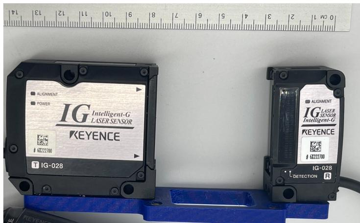
Figure 48. This shows the IG-028 T and the IG-028 R connected to the 3D printed support for proper alignment of the two component for proper reading.
