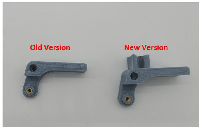
Figure 97. This shows the lever for the old extrusion system vs the lever of the new extrusion system with the protrusion to hold the perform.
