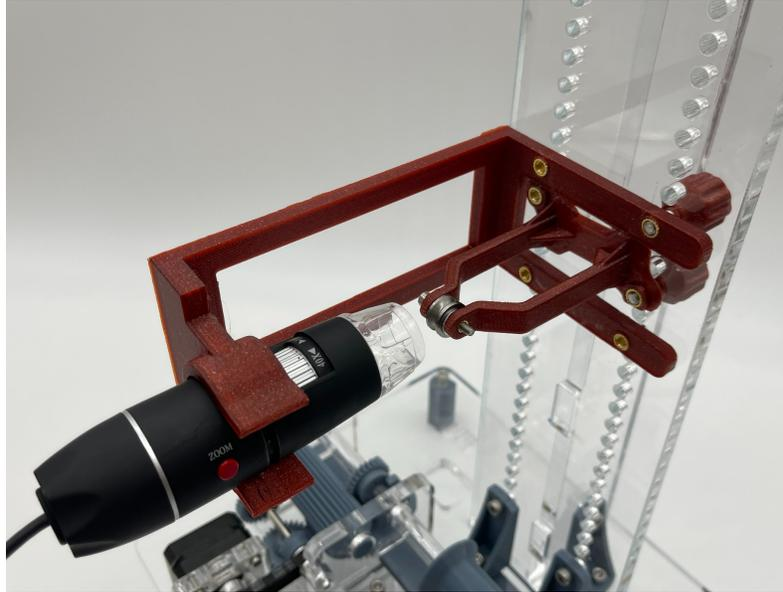
Figure 60. This shows the set up for attaining images with eh groove of the pulley as a potential background for image processing.
