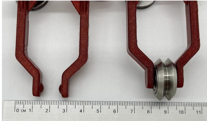
Figure 38. This is the design of the pulley support with the ball (left side) and also shows it being connected to the pulley (right side)
