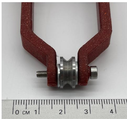
Figure 37. This is an example of the pulley when it tightly connected to the pulley support.
