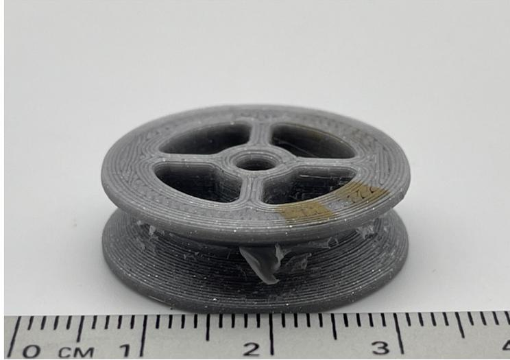
Figure 29. This shows the residual fiber left behind when it sticks on the pulley.
