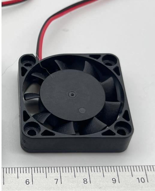
Figure 5. This is the 4010 12V DC axial fan which is was used in the cooling system for the old version of the low-cost FrED system.
