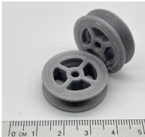
Figure 27. This is the 3D printed pulleys that was used for guiding the fiber during the drawing process in the old version of the FrED system.
