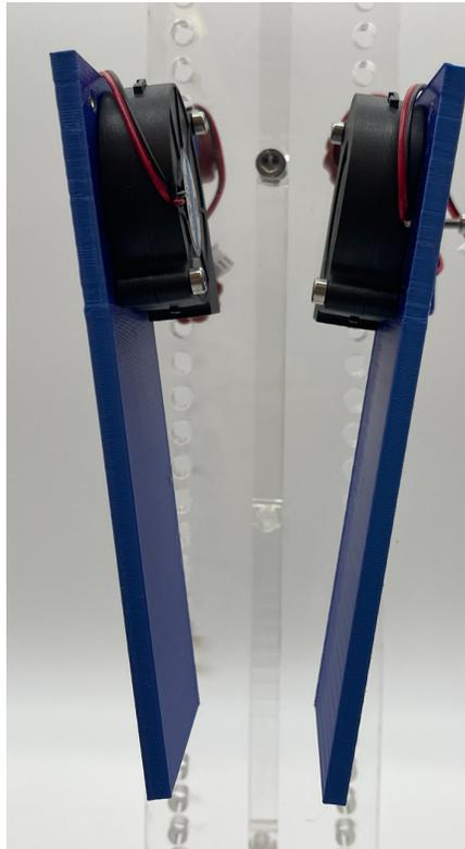
Figure 22. This is the fan frame with the hood mounted to the FrED system to enhance cooling of the fiber.
