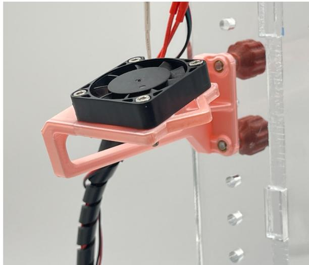
Figure 9. This is a 75-degree angled fan, and its frame is mounted on the FrED system to enhance cooling of the fiber.
