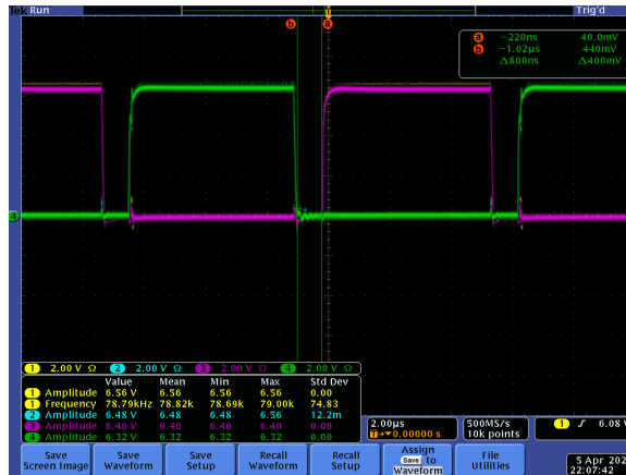
Figure B-23: 2S NCH Balancer Deadtime Verification
