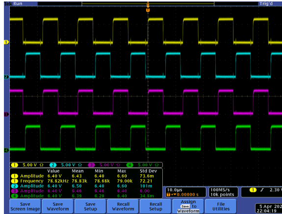
Figure B-24: 2S NCH Balancer Quasi-Synchronous Bootstrap Verification ( V_{GS} shown for each switch)
