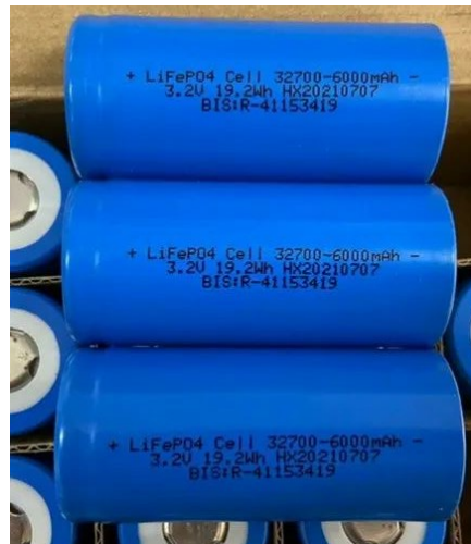
Figure 1-3: Lithium iron phosphate cell (LiFePO 4 battery)
