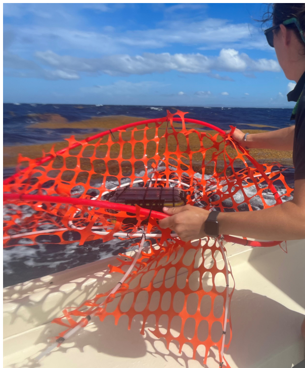
Figure 3-4: Surface drifter with partial drogue used in final deployment, with SPOT Trace GPS unit, solar panel, and lithium ion always-on battery. Noted as Drifter A in Chapter 4 .
