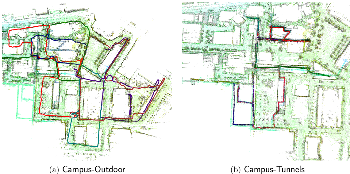
Figure 6-19: Estimated trajectories, estimated meshes, and reference point cloud for the Campus-Outdoor (6 robots, 6044m) and Campus-Tunnels (8 robots, 6753m) datasets.
