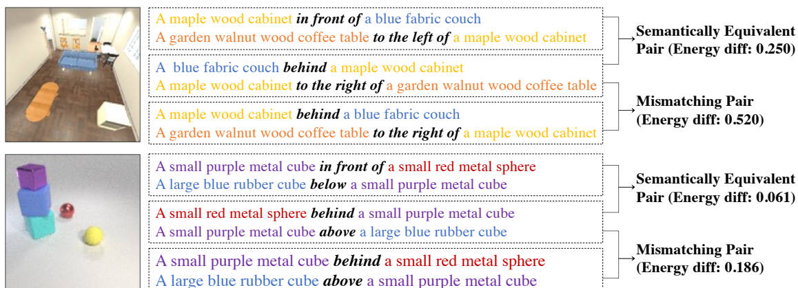
Figure 2-15: Examples of semantic equivalence on Relational CLEVR and iGibson scenes. Given an input image, our approach is able to recognize whether the relational scene descriptions are semantically equivalent or not.
