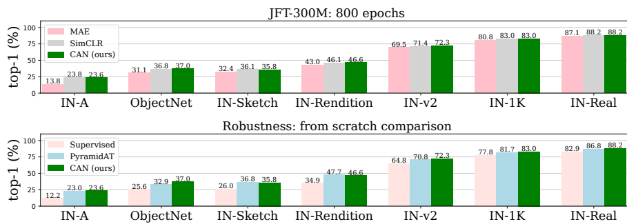
Figure D-2: Top: ViT-B models pre-trained on JFT-300M for 800 epochs, evaluated on 7 datasets with distribution shifts from IN-1K. Bottom: Comparison of our JFT-300M pre-trained ViT-B model to training ViT-B from scratch on IN-1K. We compare to standard supervised cross-entropy training with Mixup, and to PyramidAT [Herrmann et al., 2022], which uses an adversarial training method. CAN considerably outperforms supervised training, and beats PyramidAT in 6 out of 7 cases without requiring adversarial training.
