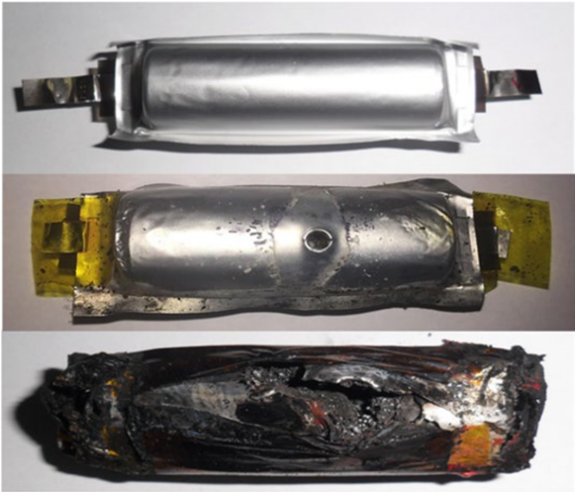
Figure 2-14: Nail penetration test for 18650 cells. Top: blank before nail test. Middle: unique electrolyte blend that is concluded to be “less explosive” Bottom: commercial carbonate-based electrolyte blend that is concluded to be “more explosive”. Reproduced from [67].
