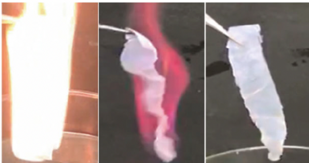
Figure 2-15: Different electrolytes subjected to a flame test, from “most flammable” on the left to “not flammable” on the right. Reproduced from [39].
