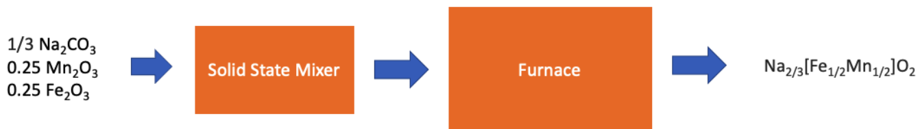
Figure 6-8: NFMO solid-state synthesis route.
