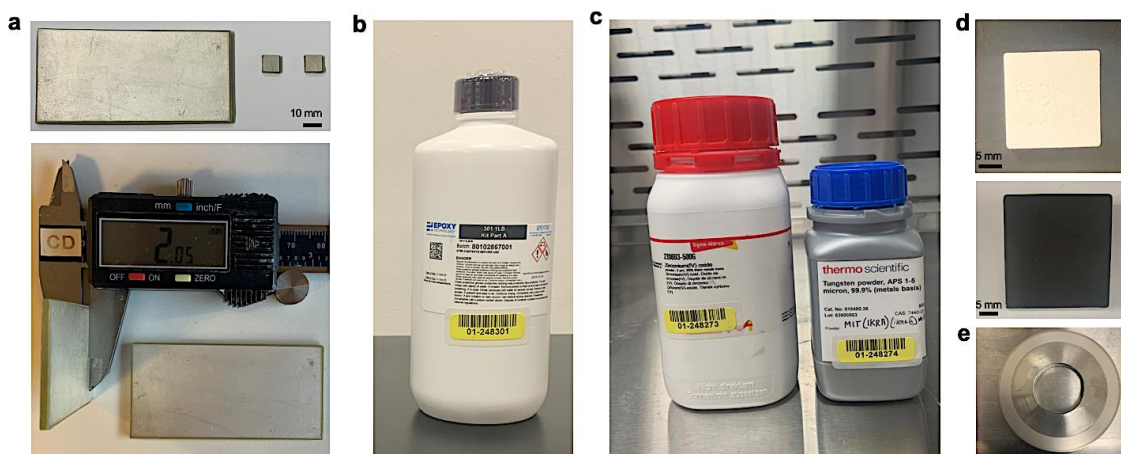
Figure 3.1: Materials used for transducer fabrication: (a) PZT bulk material diced into smaller pieces; (b) epoxy resin; (c) zirconium oxide and tungsten; (d) zirconium-load matching (top), tungsten-loaded backing layer (bottom); and (d) blade for dicing.
