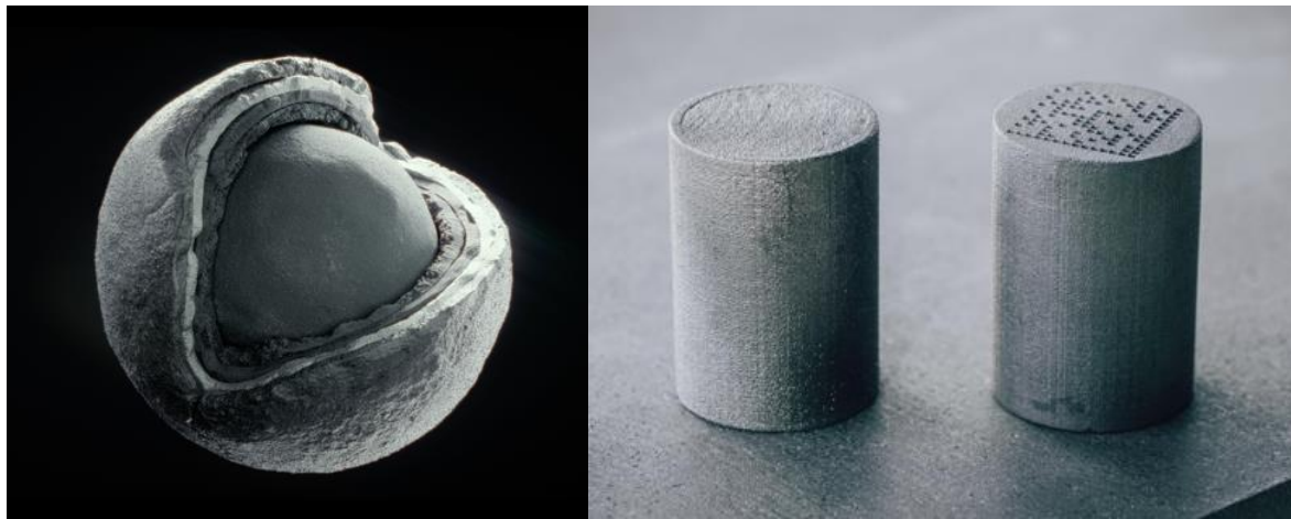
Figure 8 TRISO particle and FCM Fuel pellet from USNC, photographed by author.
