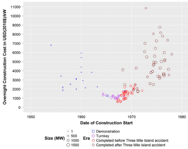
Figure 2 US Nuclear Power Reactors Overnight Construction Cost by Construction Start Date, reproduced from [21].
