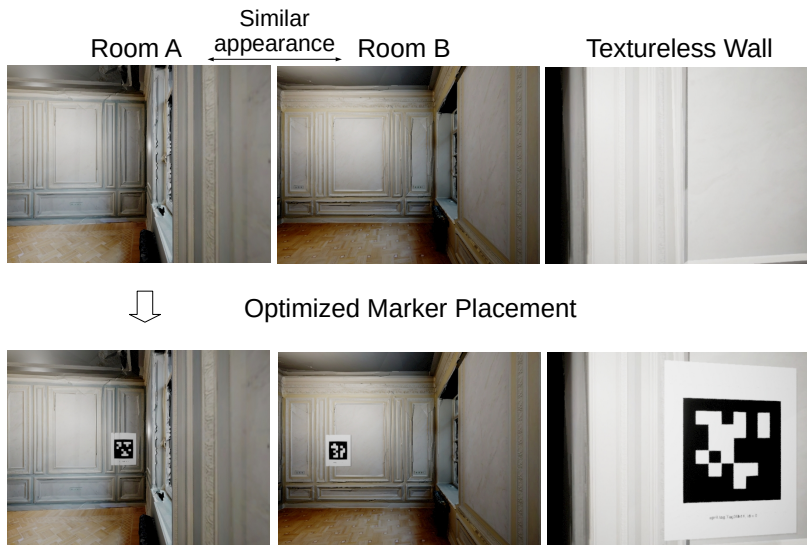
Figure 1-6: Three challenging examples for visual localization within the same scene. The images on the left and middle show two almost identical rooms in the scene, whereas the image on the right depicts a very weakly textured surface. Marker placements 1 in this scene guided by our optimized marker placement approach led to improved visual localization on these examples.
