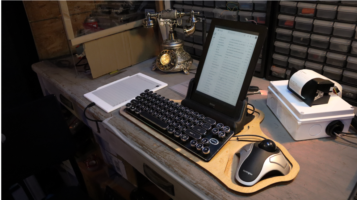
Figure 8-1: All of my asynchronous communication is designed to happen at this desk—texts are handwritten on the tablet (and automatically sent once written), incoming texts are printed, phone calls are routed through the rotary phone, and email happens on the main typewriter-like interface with an e-ink screen.
