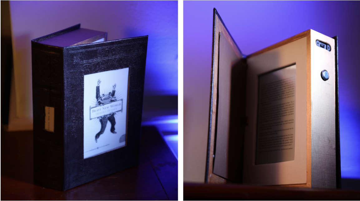
Figure 7-1: The Huxley Smart Book, showing updating e-ink displays on the cover, spine, and inside. A USB port on top is available for charging, one button is available for turning pages. Huxley only updates when the user is away and the current book has been completed or ignored. Its selection is based on the measured interests and affective state of the user at work.
