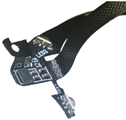
Figure 5-17: Pre-bent Flex Circuitry
