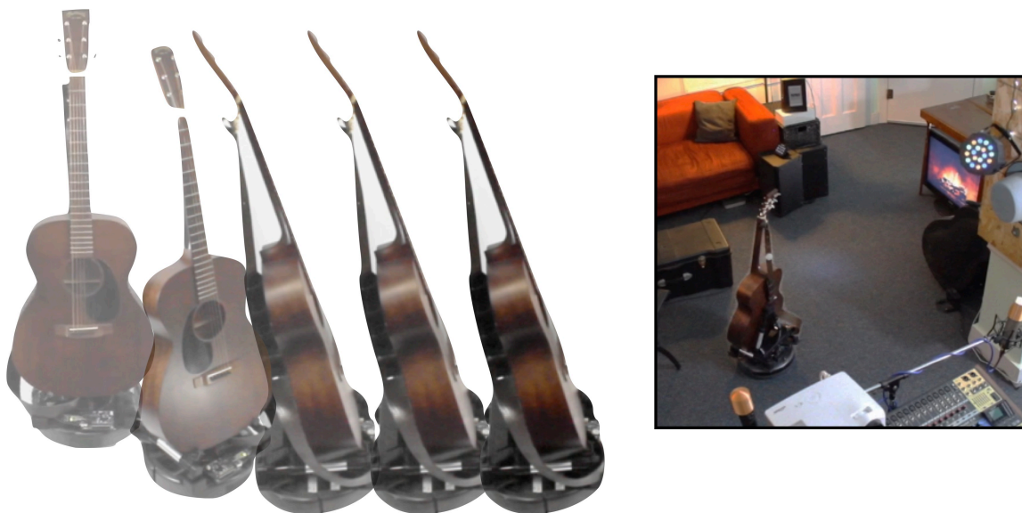
Figure 7-2: Guitarbot is a guitar stand built on top of a iRobot Create 2, that can rove around the space and find the positions most likely to result in guitar use.
