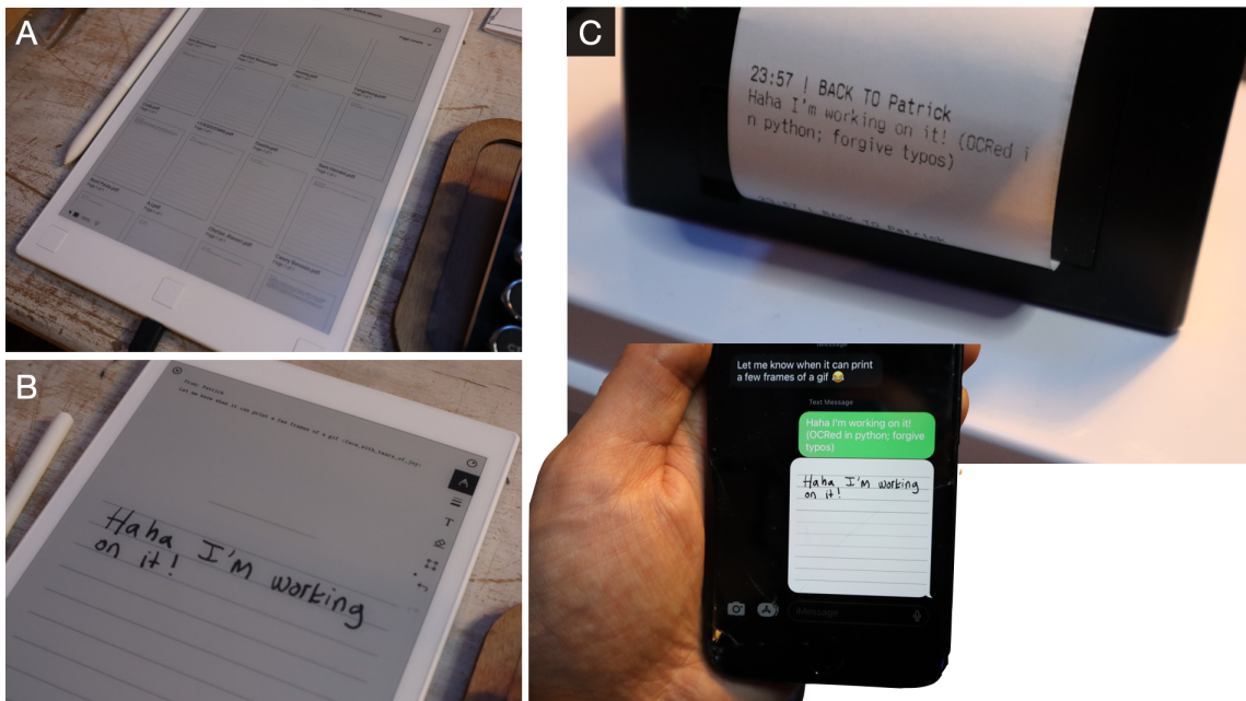
Figure 7-8: To send texts, the user selects one of the auto-generated documents that correspond to every incoming texts, sorted chronologically (and seeded with everyone in the address book) [A]. After clicking on a document name (labeled by sender) the user handwrites a reply [B], which automatically gets OCRred and sent in both text and image form. Upon success, it is also printed to the receipt printer [C].
