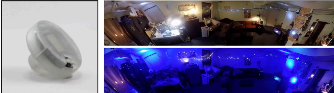
Figure 7-3: Stagehand marries a custom button which attaches to the guitarstrap (left) with an immersive living room system (right). Whenever the guitar is lifted and in use, the entire environment shifts to 'concert mode' (right bottom).
