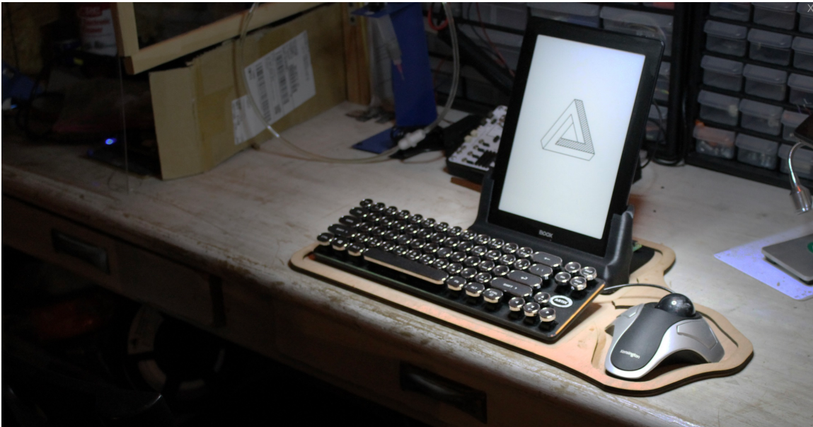
Figure 7-5: This email device is an e-ink screen VPned to a small single board computer (latte panda); designed to evoke a typewriter and to feel different than a typical laptop.
