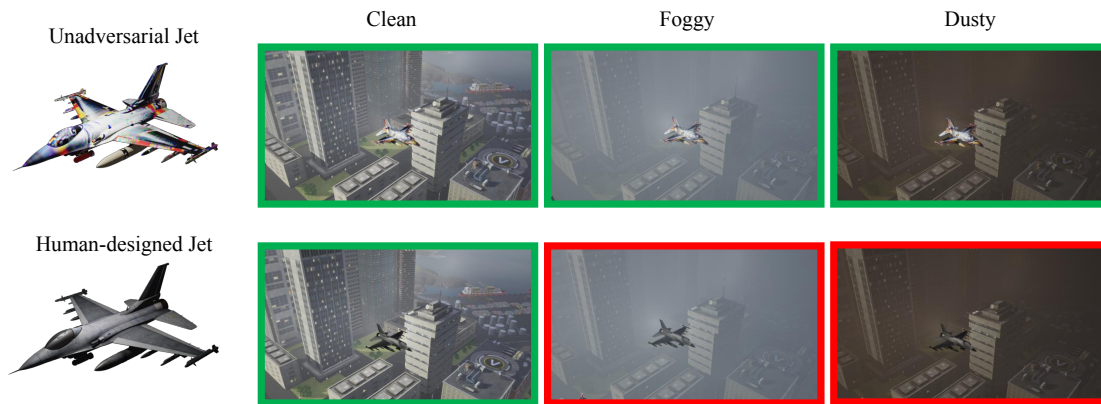
Figure 3.1: We demonstrate that optimizing objects (e.g., the pictured jet) for pre-trained neural networks can boost performance and robustness on computer vision tasks. Here, we show an example of classifying an unadversarial jet and a standard jet using a pretrained ImageNet model. The model correctly classifies the unadversarial jet even under bad weather conditions (e.g., foggy or dusty), whereas it fails to correctly classify the standard jet.
