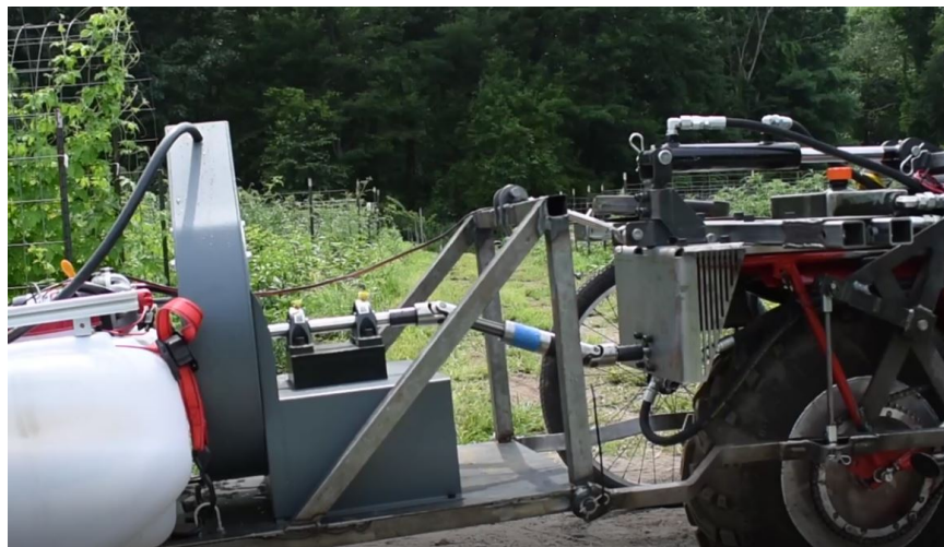
Figure 2-7: The Bullkey PTO spindle connected a rear-mounted implement.
