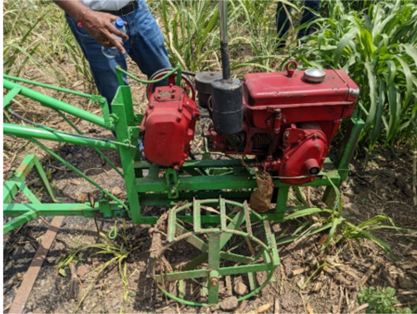
Figure 1-2: A jugaad tractor equipped with blade harrow.
