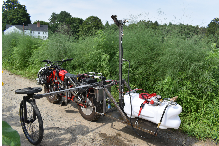
Figure 2-11: Prototype vertical sprayer mounted on the Bullkey tractor.
