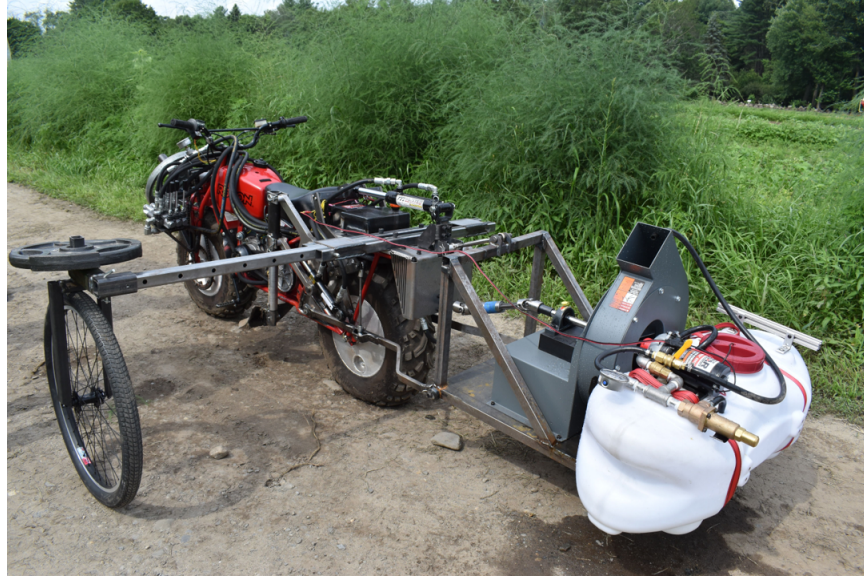
Figure 2-10: Bullkey supports the blower and 15ga water tank via 3pt hitch. The PTO is connected to the blower via universal link.
