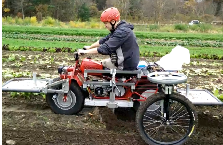
Figure 1-5: A test-rider operates the original Bullkey vehicle side-saddle. The height control prevents them from straddling the vehicle.
