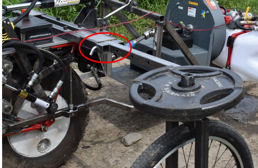
Figure 2-1: A closeup of the outrigger wheel. The pin which fixes the length is circled in red.
