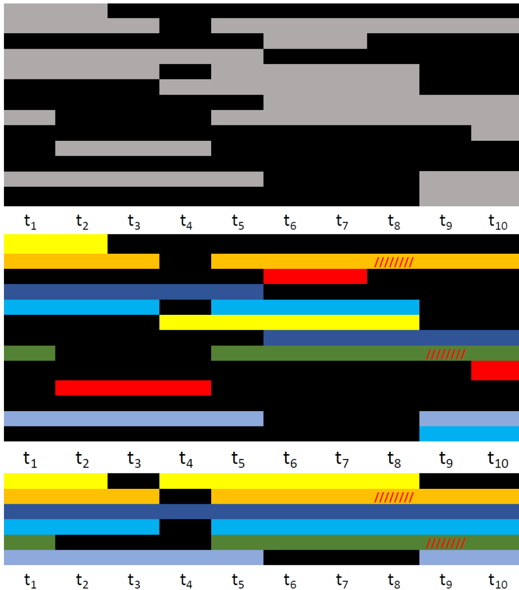
Figure 3-2: Showing the two key steps of SOMA. The inputted data is formed of many disjoint tracklets, visualized in the top section in grey. The x-axis represents time, and the y-axis represents tracklets of markers. In the first step, the matching tracklets are identified. This is visualized in the middle section, where matching colors are applied to different tracklets which represent the same marker. Then, these matching tracklets are combined robustly to handle occlusions. Gaps in the tracklet data are representative of occlusions (no data recorded). The final step involves assigning a label name to each marker for the part of the body (not pictured). Figure from the SOMA paper [2].
