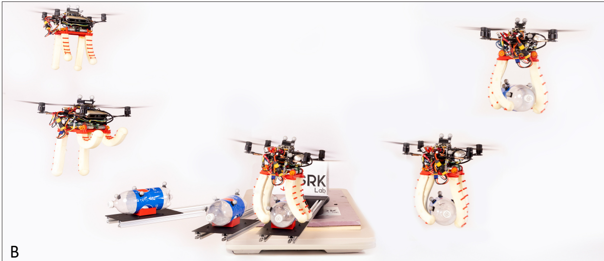
Figure 2.6: Timelapses of experiments with moving targets. (A) Moving grasps of med-kit attached to a quadruped robot that has forward velocity of 0.3 m/s and with a relative grasp speed of 0.1 m/s. (B) Moving grasps of two-liter bottle on a turntable moving with a tangential speed of 0.08 m/s and with a relative grasp speed of 0.5 m/s; see Movie 1 for more visualizations.
