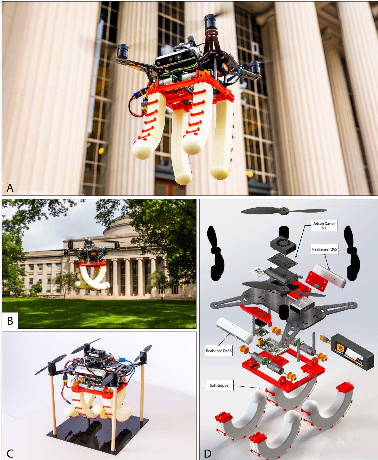
Figure 1.1: Overview of the Soft Drone. (A-B) The proposed Soft Drone platform flying outdoors. (C) Front view of the Soft Drone platform, with the soft gripper in the passively closed state. (D) Exploded CAD view of the quadrotor and gripper, including onboard sensing and computation.
