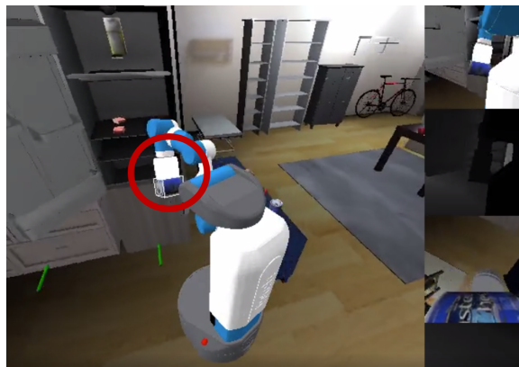
Figure 2-4: This figure depicts the Fetch robot grasping a can (in red) in the Habitat simulator.
