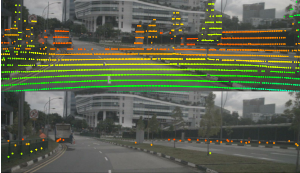
Figure 3-2: Radar returns are far sparser than LiDAR point clouds.
