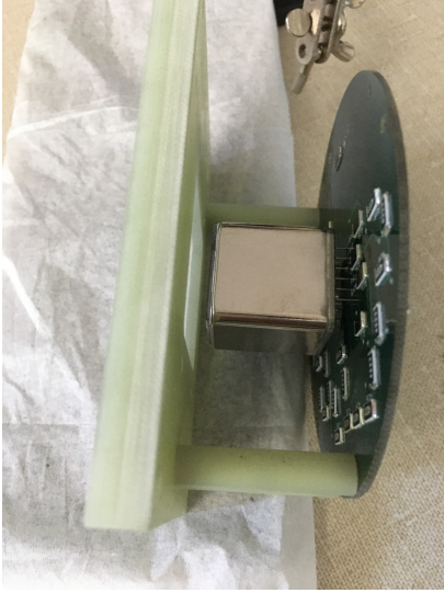
Figure 7-4: Two of the veto PMT assemblies constructed at MIT, including the 1-inch PMT, base circuit board, and TPB-coated acrylic window.
