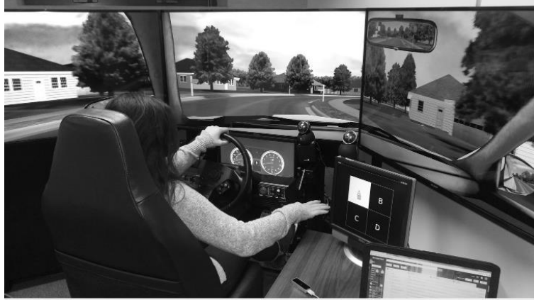
Figure 2. Driving simulator setup, visual display monitor with webcam, and LEAP Motion
