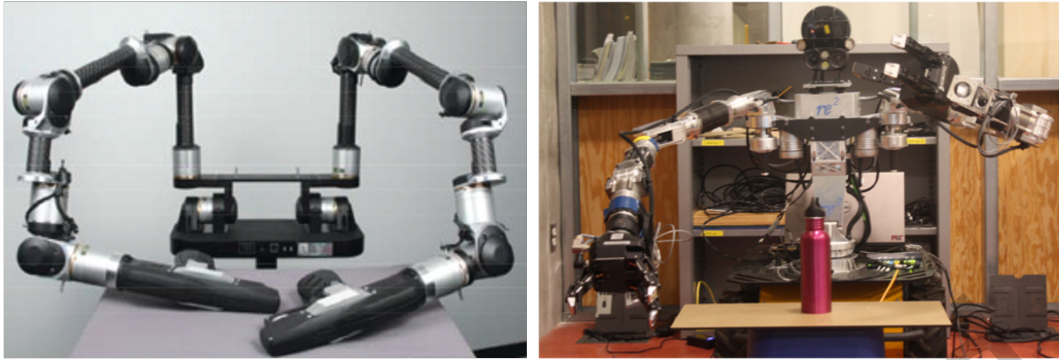
Fig. 1. Robot hardware used during the user study. Left : Imitation Controller (IC), a passive device used for teleoperation. Right : Robot for bimanual manipulation, including two 7-DoF arms, 2 grippers and on-board 2D&3D sensing. The IC is a scaled kinematic replica of the robot, enabling direct teleoperation (A & B) by commanding the robot to follow the joint angles of the IC on-line. For the teleautonomy conditions (C & D), the robot is commanded from a computer-based user interface.
