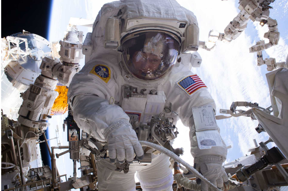
Figure 1.2: Astronaut Peggy Whitson on an ISS EVA in 2017. Note her left wrist, which sports a printed EVA timeline with notes about the tasks the crew needed to perform. Credit: NASA (source).
