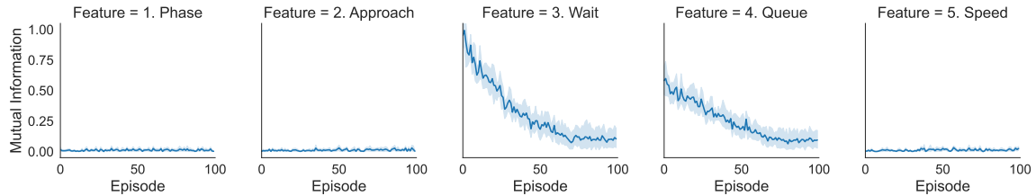
Figure E-2: Masking the number of vehicles approaching and the average speed in the 7-intersection use case. Evolution of the Mutual Information between the reward and each of the five features considered in the RESCO benchmark for Traffic Signal Control during learning. The mean and 95% CI across 7 intersections is shown.
