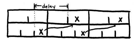
In the diagram, we have shown two arriving frames and the corresponding departing frames. (The departing link has a lower raw bit capacity so slots are wider, but all slots contain b bits.)
