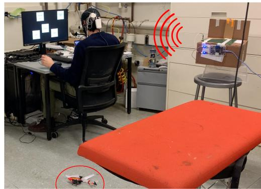
(b) In the second part of the experiment, the SDR hacking was turned on (top right), which activated the Emergency stop command. Consequently, the drone crashed to the ground (bottom left).
