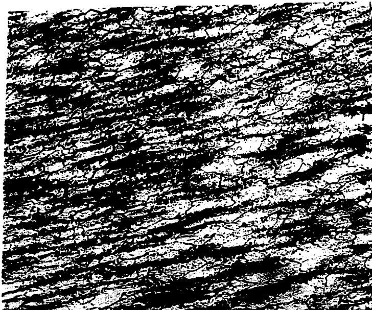
Figure 15. Modified H.S. 21 hot worked at 1150°C, cold rolled to 15.2% RA. 5% HCl electrolytic etch. 158X.
