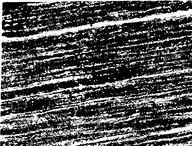
Figure 47. Modified H.S. 21. Hot worked at 1150^{\circ}\text{C} , cold rolled to 11.1% RA, heat treated at 1065^{\circ}\text{C} for 12 minutes, air cooled. 5% HCl electrolytic etch. 158X.
