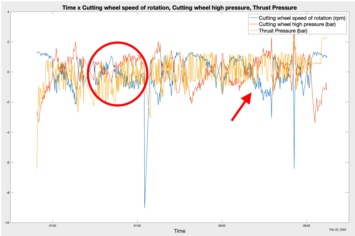
(b) Ring 598: Rock-like mixed. Here a lot of variation can be observed, especially in thrust pressure. The red circle and arrow indicate regions where there is positive and negative correlation between cutting wheel speed of rotation and cutting wheel high pressure.
