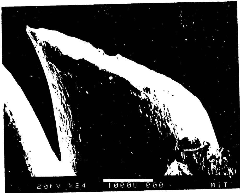
Figure 18 - Low-magnification view of the shear-instability tensile fracture.
