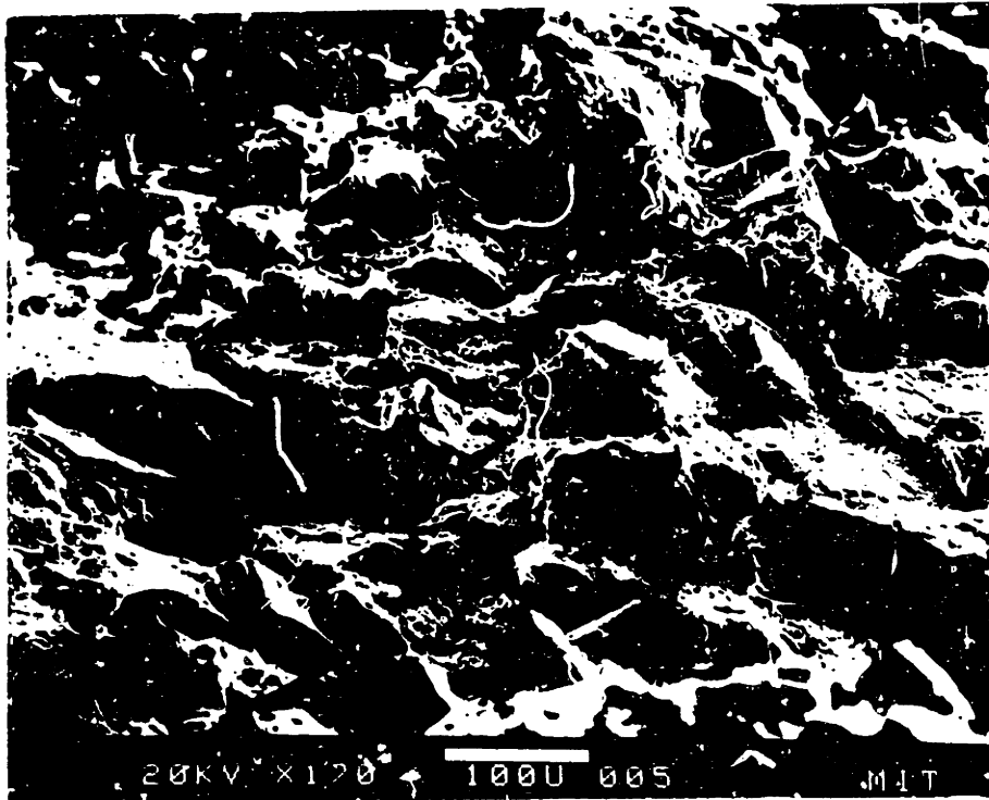
Figure 23 - SEM fractograph of 26Ni-4Cr(H) tensile tested at -55°C showing some intergranular fracture.
