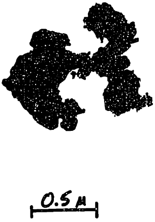
Figure 4.5 TEM micrographs of Baikowski mullite, 3\text{Al}_2\text{O}_3 \cdot 2\text{SiO}_2 .
