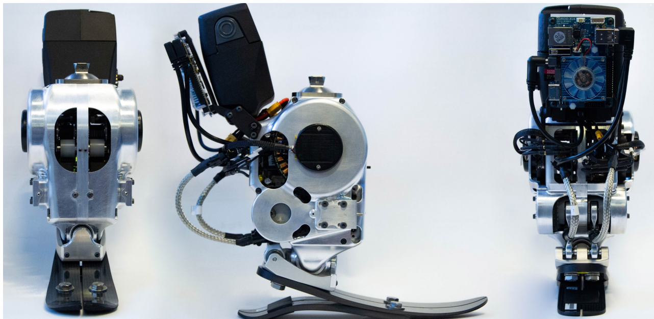
Figure 1. Overview of the 2-DoF ankle prosthesis, which is designed for untethered mobility, tailored for individuals around 75 kg, and suitable for varied terrains.
