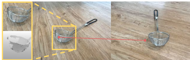
Fig. 3: Baselines. Multi-view Stereo represents a potential alternative to depth cameras. However, the depth maps estimated by COLMAP (a widely-used MVS method) [16] exhibit significant artifacts on thin or reflective objects, which leads to incorrect correspondences between pixels (shown in red).
