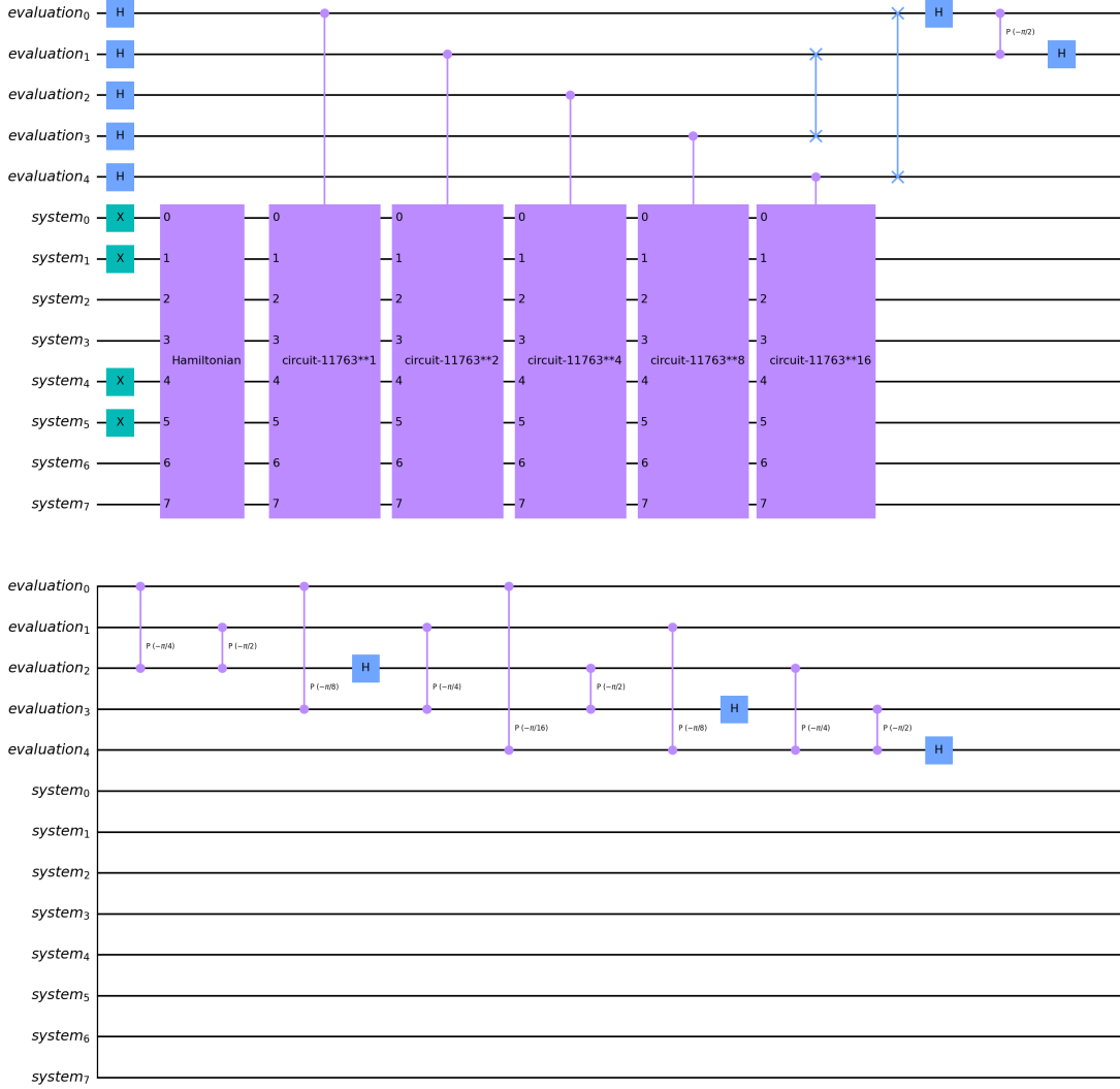
Figure D.6: A QPE circuit with for H_4 molecule, where a Hartree-Fock initial trial state preparation circuit is also showed at the beginning. The circuit block labelled as "Hamiltonian" after the four initial Pauli X are a basis transformation unitary from canonical MO basis to localized orbitals (LOs).
