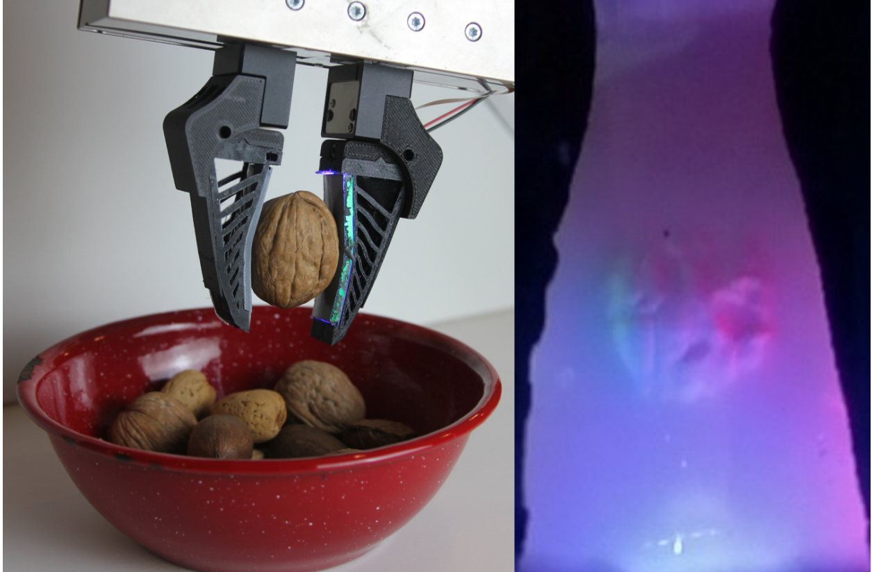
Figure 5.1: The Baby Fin Ray grabbing a walnut (left) and the corresponding cropped raw image of the mirror that displays the tri-colored tactile sensing region and the indentation of the walnut shell (right) [15].
