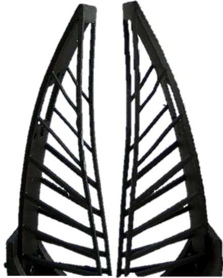
Figure 8.3: The Onyx-based Fin Ray. The struts were thinned down and made narrower to help the structure deform, but the resulting structure still had signs of plastic deformation after a single grasp, which is shown in the curved struts and “tactile” section.
