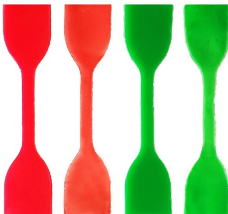
Figure 5.6: Fluorescent silicone paint dogbone samples used for tensile testing on the Instron meeting. From left to right, we have our pink Silc Pig, pink synthesized paint, green Silc Pig, and green synthesized paint samples [15].
