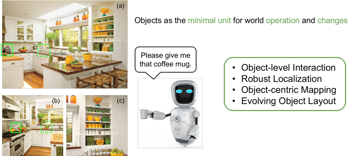
Figure 1-1: Object-level reasoning is a desirable capability for advanced robotic tasks where traditional SLAM approaches are not a perfect fit. For a robot operating in a household environment (a) with an object retrieval task, it is expected to develop a sense of “objectness” in the environment, e.g., coffee mugs on the shelf (c), and keep up with the evolving object layout of the room (b).
