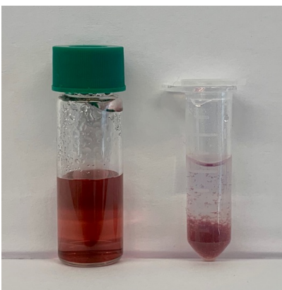
Figure 3-1: Prepared samples of AuNP-CysAA solutions in a 4 mL glass vial (left) and a 2 mL centrifuge tube (right).
