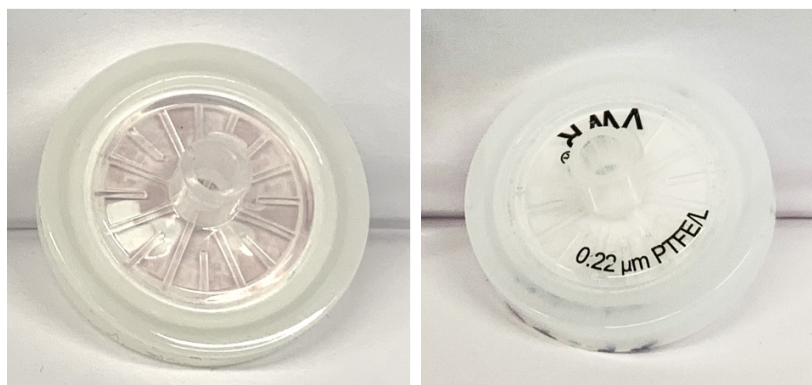
Figure 3-11: 25 mm PES syringe filter (left) and 25 mm PTFE syringe filter (right). The PES is noticeably stained with AuNPs that stuck during recovery.
