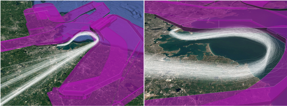
Figure 2-26: The magenta volume highlighted represents the combined volumetric airspace constraints affecting a westbound departure procedure from runway 22R. They include airspace reserved for arrival and approach procedures, airspace reserved for the final approach controller, and airspace reserved for the south sector controller.
