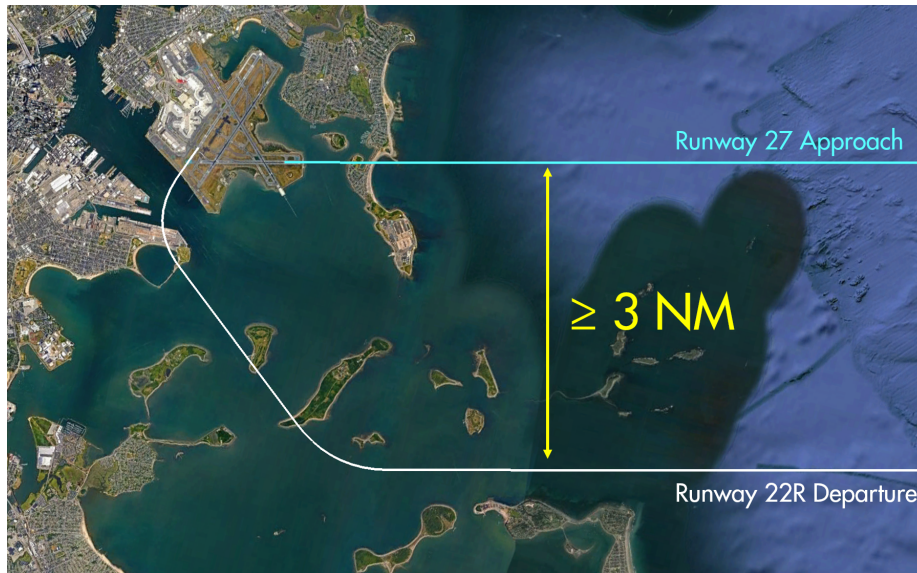
Figure 2-5: Example of lateral separation being prioritized in the design of flight procedures, due to aircraft vertical profiles not being controlled to the same extent as their lateral profiles.
