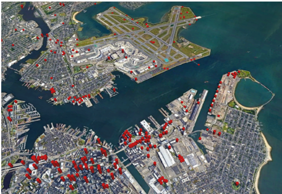
Figure 2-13: Red cylinders indicate ground obstacles as recorded in the FAA's DOF database for the Boston area.
