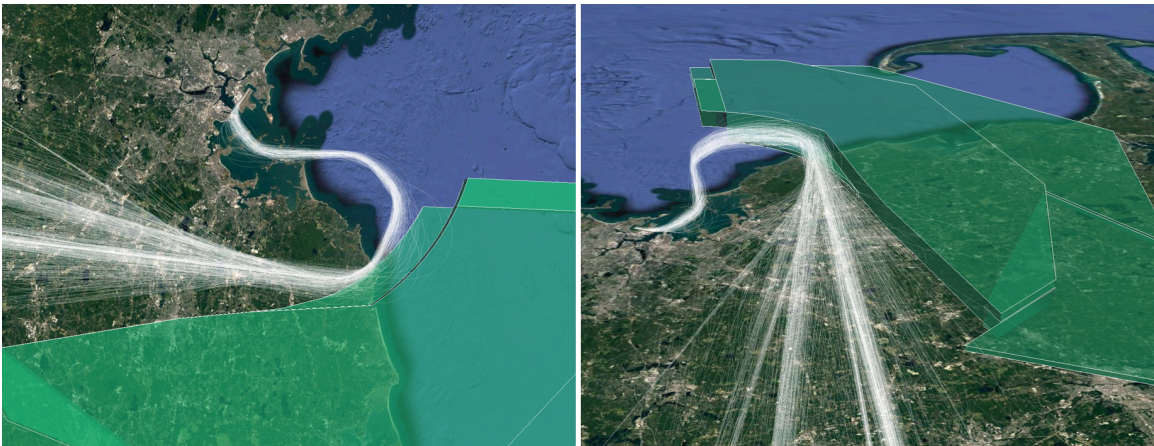
Figure 2-23: The green volume highlighted represent airspace unavailable to a westbound departure procedure due to it being allocated to southbound operations. The white tracks represent current aircraft trajectories on westbound departures off runway 22R.
