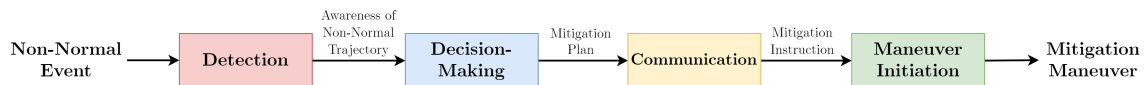
Figure 4-15: The mitigation process can be parsed into four distinct functions: detection, planning and decision-making, communication, and maneuver initiation.
