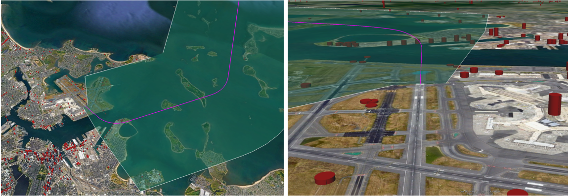
Figure 2-14: Illustration of the Obstacle Clearing Surface (OCS) in green for a departure procedure off runway 22R at BOS, drawn based on TERPS criteria. Obstacles are shown as red cylinders.
