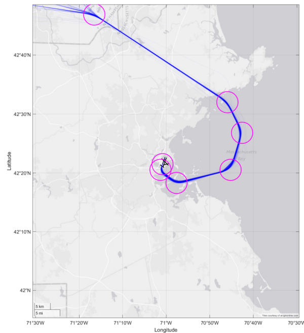
Figure 4-9: Flight tracks of aircraft tracking the HYLND RNAV departure procedure from runway 22R at BOS. Magenta circles represent 1.5 NM distance rings around each procedure waypoint.
