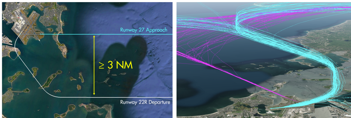
Figure 6-10: Left: Lateral procedure tracks for the RNAV departure from runway 22R (white) and ILS approach to runway 27 (cyan). Right: Example radar tracks of aircraft tracking both procedures. The higher dispersion in vertical profiles on the RNAV departure can be observed.
