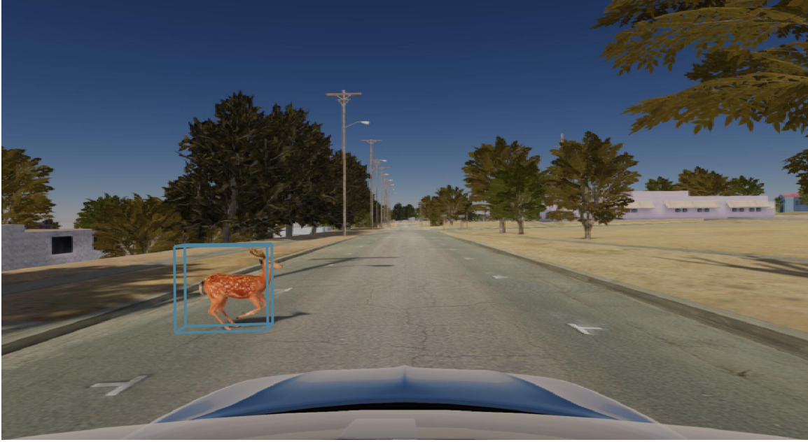
Figure P-3: Camera Image for the scenario in Fig. P-1. Blue bounding box is the ground truth detection. The camera fails to detect the deer crossing the road (mis-detection failure).
