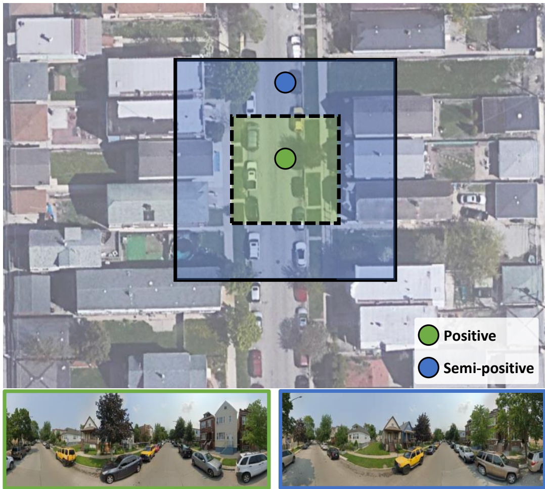
Figure 3-2: Positive pairs vs. semi-positive pairs. For the satellite image outlined in solid black, a ground image taken in the green shaded center region (ground image shown outlined in green) makes a positive pair and a ground image taken in the blue shaded region (ground image shown outlined in blue) makes a semi-positive pair. Previous works only match between positive pairs.
