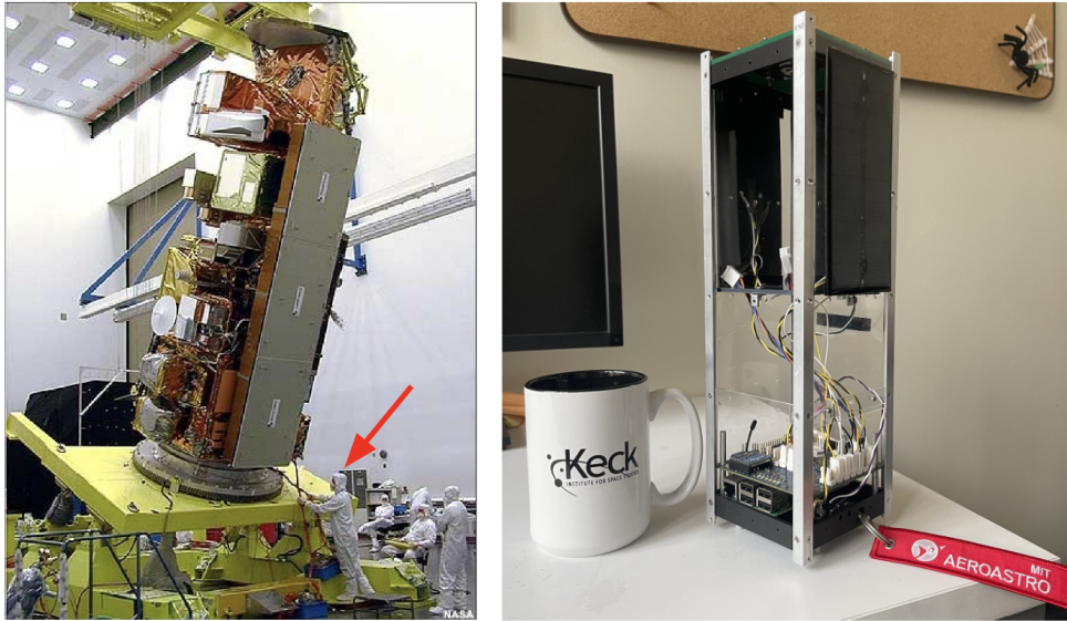
Figure 1.6: size Comparison of ESA’s EnviSat (left) with human for scale (image courtesy of ESA) and a 3U ( 10 \times 10 \times 30 \text{ cm}^3 ) nanosatellite model (right) with coffee mug for scale. Model courtesy of Paul Fucile from WHOI.
