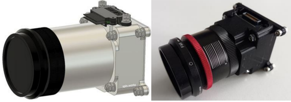
Figure 3.11: The AEROS HSI payload assembly developed by Spin.Works [50].
